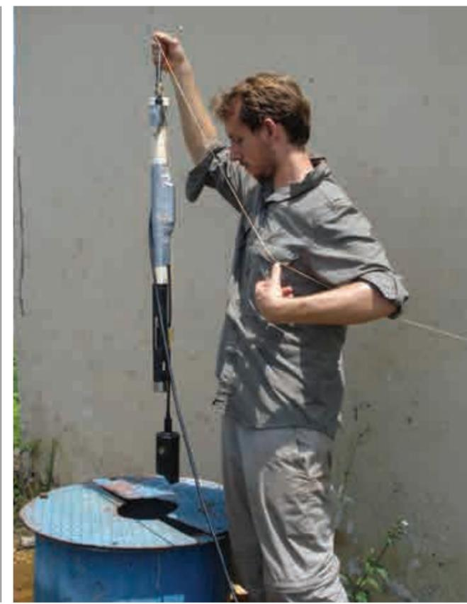
The tryptophan sensor is quick, reagentless, and cheap, so it can enable rapid surveys of dozens of wells and boreholes across the town.
