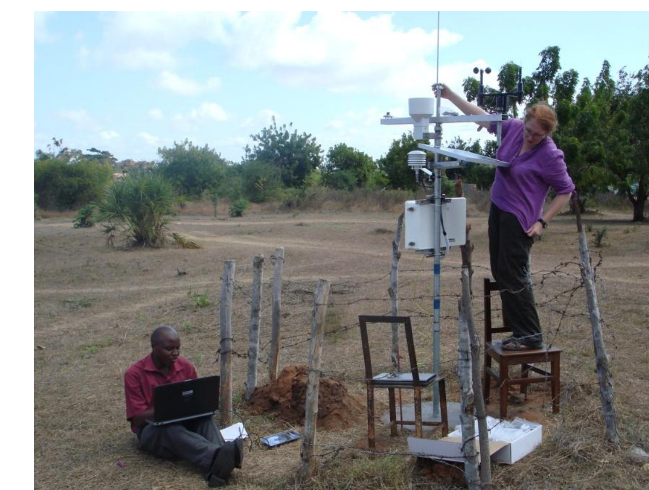
Figure 5: Weather station installation in Kilwa
