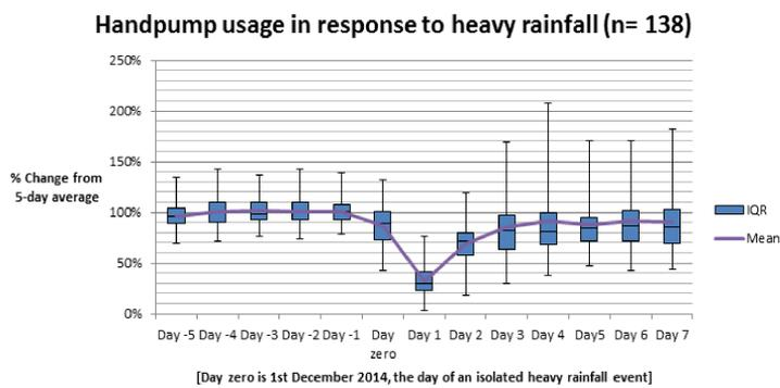
**Figure 2.** This diagram shows the handpump usage immediately before and after an isolated day of heavy rainfall on December 1<sup>st</sup> 2014 (n= 137).
