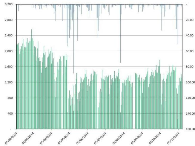
**Figure 1.** This figure shows how community pump usage (litres per day, in green, left hand y-axis) varies over the year in response to rainfall (mm blue, right hand y-axis) in 2014. [The zero periods in May and August represent network outages.]
