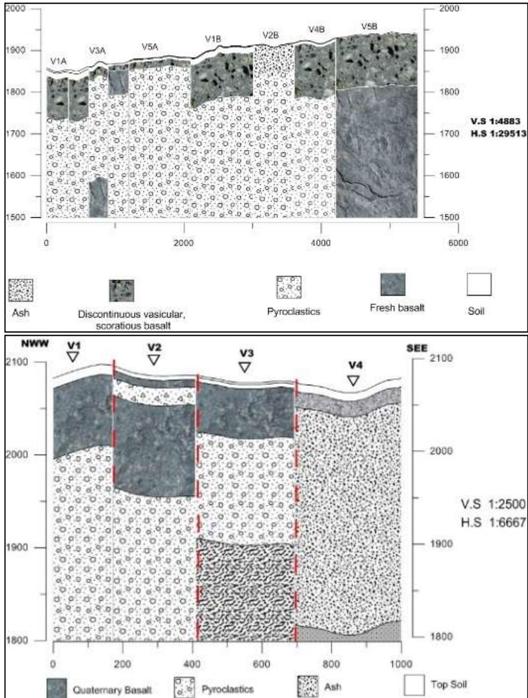
Figure 3: Local variations of subsurface geology as represented by geoelectric sections of volcanic and pyroclastic rocks in the study area
