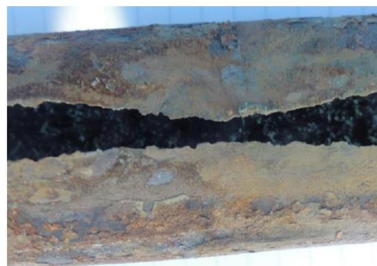
**Photograph 2. Perforation of a rising main from corrosion**
